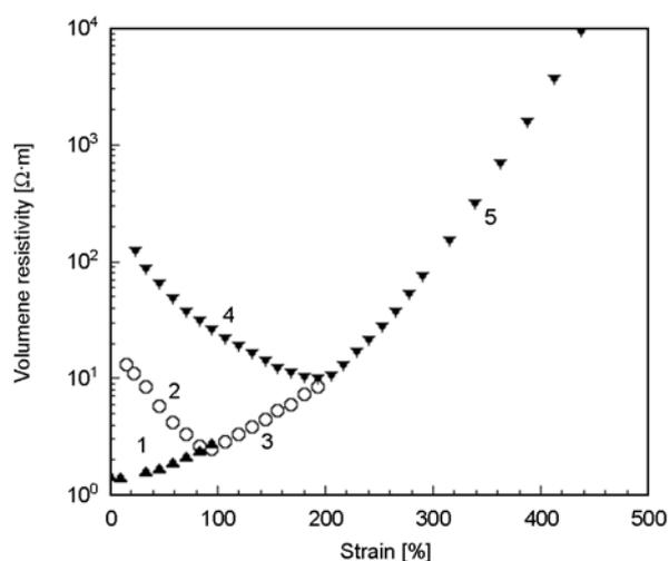
**Figure 3.** Strain dependence of the electrical resistivity for NR filled with 3 phr of MWNTs
