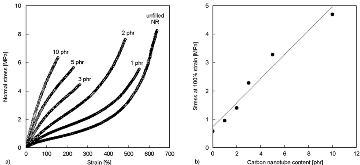
**Figure 6.** Stress-strain curves (a) and stress at 100% for pure NR and MWNTs composites (b)
