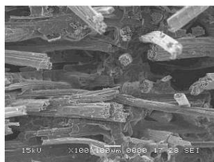
**Figure 8.** Cross section of untreated jute reinforced PP
